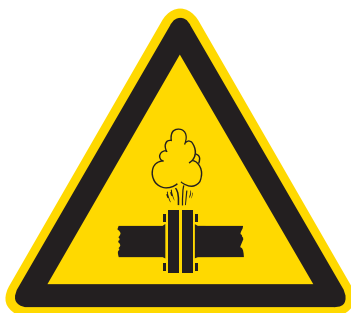
W80... Warning of over pressure
