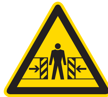
W23... Warning of Squashing hazard, BGV A8 W23, DIN 4844-2 D-W023
