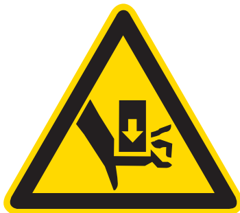
W73... Warning of squashing hazard by pressing tool
