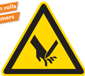
W57... Warning of cutting injury
