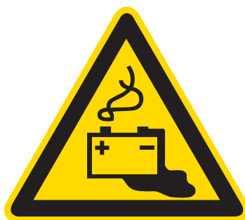
W20... Warning of leaking batteries, BGV A8 W20, DIN 4844-2 D-W020
