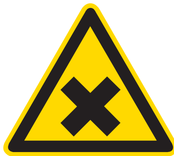
W18... Warning of harmful or irritant materials, BGV A8 W18, DIN 4844-2 D-W018
