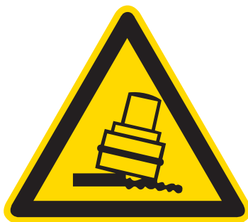
W24... Warning of the danger of tipping rolling, BGV A8 W24, DIN 4844-2 D-W024
