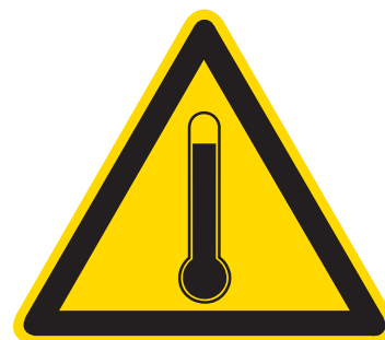
W86... Warning of high temperature
