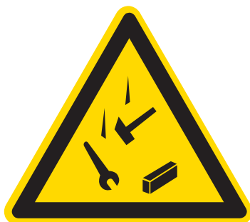
W35... Warning of falling objects
