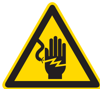
W51... Warning of dangerous electrical voltage
