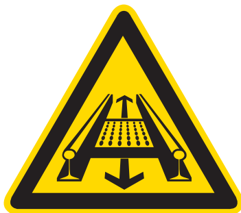
W29... Warning of danger by a conveyor in track, BGV A8 W29, DIN 4844-2 D-W029
